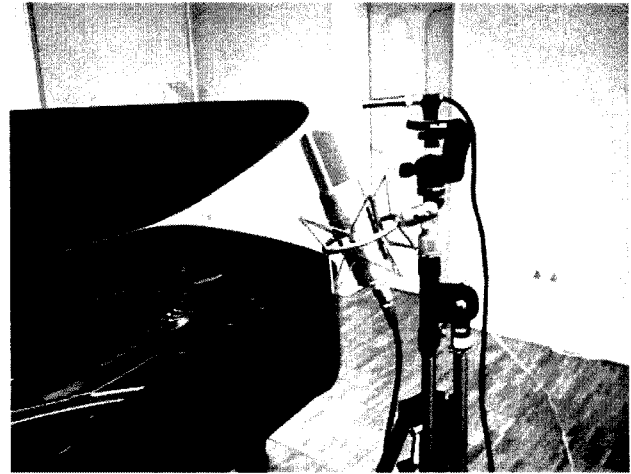
Fig. 1 Setting of a Steinway and Sons model D grand piano and microphones used for recording and peak level monitoring.
