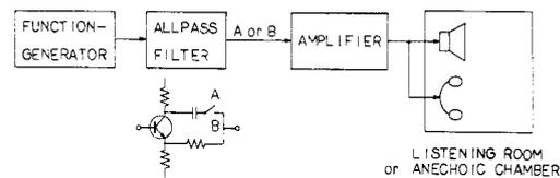
Fig. 6. Schematic diagram of instrumentation.
