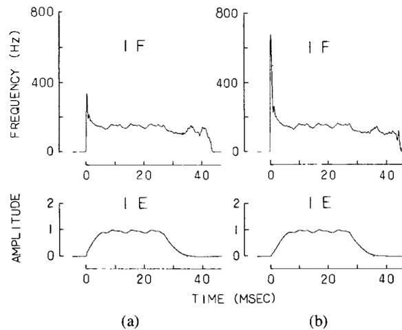
Fig. 11. Instantaneous frequencies (IF) and instantaneous envelopes (IE) for headphone listening. (a) unfiltered S2. (b) filtered S2.
