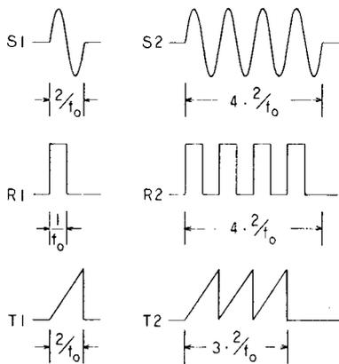
Fig. 4. Transient signals used for hearing test.
